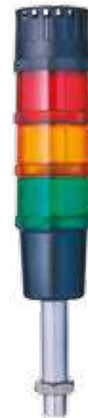
Order number: C70-Q641 Colours: red/orange/green Function: LED steady beacon, buzzer steady or pulsing tone Nominal voltage: 24 V AC/DC Type of mounting: horizontal Length: 100 mm
