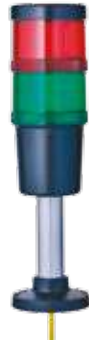
Order number: C70-Q02 Colours: red/green Function: LED steady beacon Nominal voltage: 24 V AC/DC Type of mounting: horizontal Length: 100 mm
