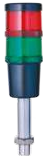
Order number: C70-Q602 Colours: red/green Function: LED steady beacon Nominal voltage: 24 V AC/DC Type of mounting: horizontal Length: 100 mm
