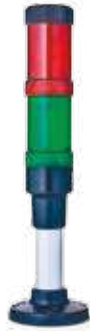
Order number: ECO40-Q02 Colours: red/green Function: LED steady beacon Nominal voltage: 24 V AC/DC Type of mounting: Tube mounting (100 mm tube length)
